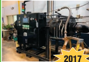
Atmosphere Engineering A11636 Exothermic Generator
