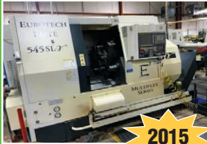
Eurotech Elite B545-YS CNC Turning Center
